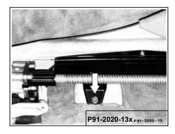
6 Unscrew screw (1 each) on left seat rail (arrow).
