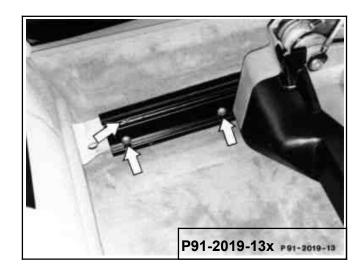
3 Unscrew screws (2 each) at rear on right seat rail.
