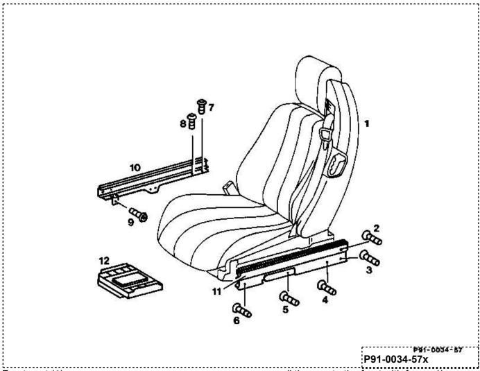
Front seat (1) move all the way to the front with forward/ backward adjustment mechanism. Screws (2, 3, 4, 7 and 8) (5 each) unscrew on rear of seat rail at left and right. 17 Nm.
