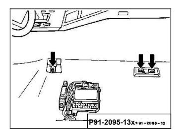
Seat mounting points on floor assembly - tunnel area.
