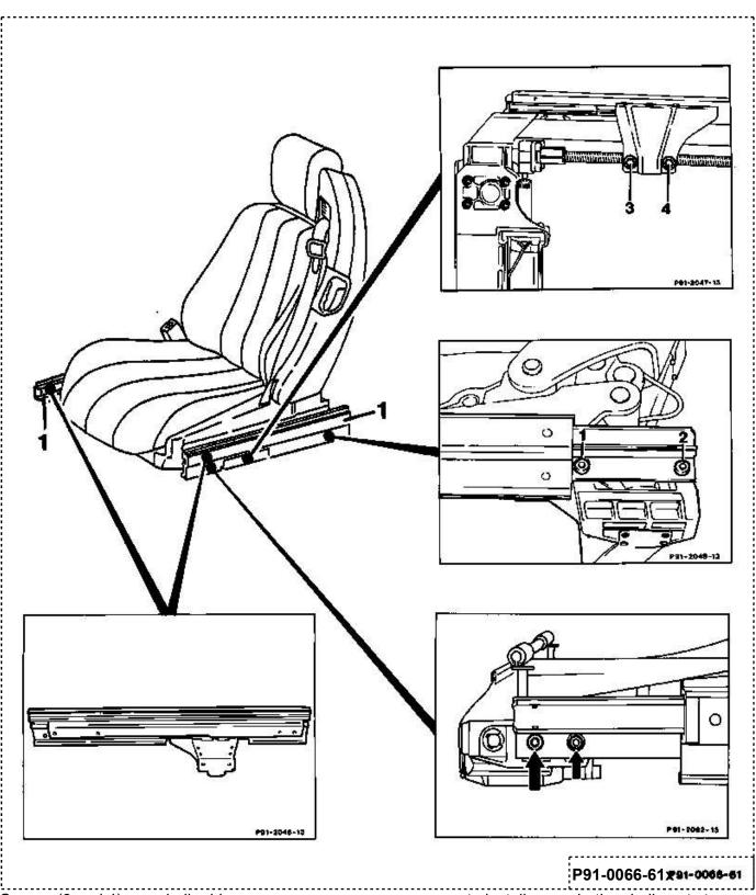
Screws (3 and 4) on spindle drive...... unscrew, to install screw both spindle nuts to rear end stop. 25 Nm.
