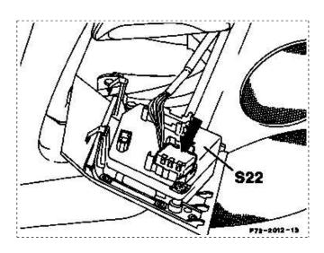
10 Screw out screw on inside door control (arrow).
