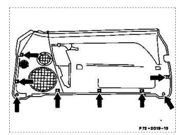
Rear side of door liner showing position of clips (8 each, arrows).
