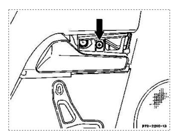
8 Press large wood cover downward and remove from door liner (arrows).
