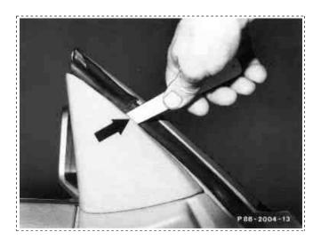
4 Press off small wood cover and knob for inside locking mechanism and remove (arrows).
