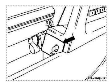
6 Pull out entry light downward. Disconnect electrical connections and lay light aside.
