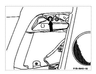
11 Screw out screw at front of door pocket (arrow).
