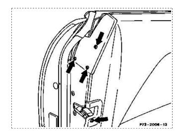
3 Press cover off of mirror triangle and remove upward.
