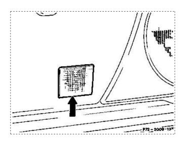
7 Screw frame off of inside door control and remove (arrow).
