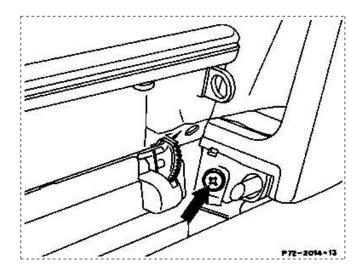
12 Screw out screw at rear of door pocket (arrow).
