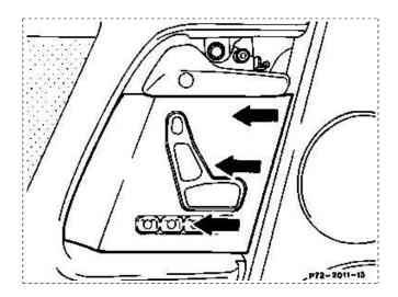
9 Disconnect plug connector and lay wood cover to side (arrow).
