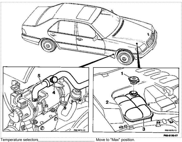
Sealing cap (1) on coolant expansion
