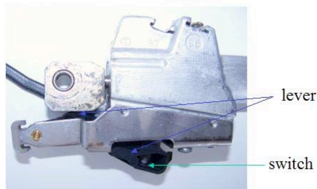
As the cylinder rod retracts, the top piece moves a lever that releases the micro switch.
