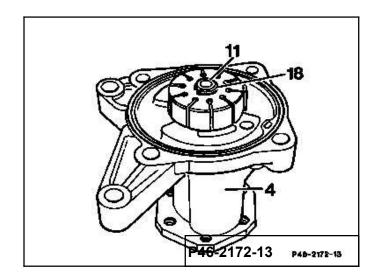
20 Insert the cam insert with the cast or stampedin direction of rotation arrow (arrows) facing upwards into straight pins on the pump housing.
