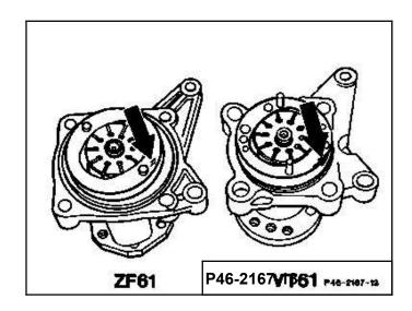
21 Insert vanes (10 off) into the rotor with the rounded, metallic glossy sides (arrow) facing the cam insert.
