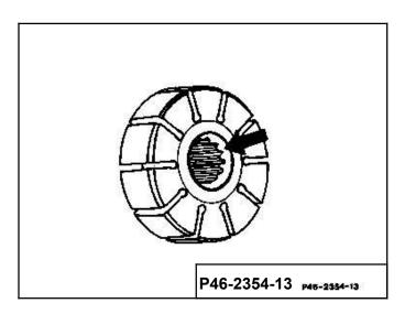
37 Install new locking ring (18). The locking ring (18) must be correctly seated in the groove of the drive shaft.
