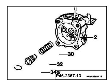
27 Press in radial seal ring (28) as far as the stop with a suitable mandrel.
