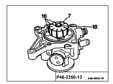
38 Insert vanes (10 off) into the rotor with the rounded metallic glossy sides (arrow) facing the cam insert.
