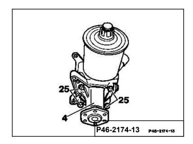
24 On the Vickers/LUK power steering pump, insert new O-ring, then fit on reservoir (35) and attach with the bolts.
