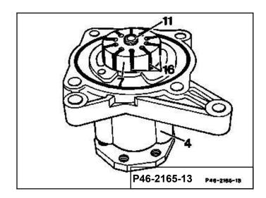
8 Remove drive shaft (11) from the bearing flange (4).
