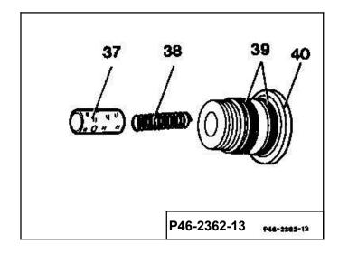
34 Screw all 4 screw cartridges (40) into the housing in the consecutively numbered order shown in number 10, 40±5 Nm. Use pronged wrench 129 589 02 07 00.
