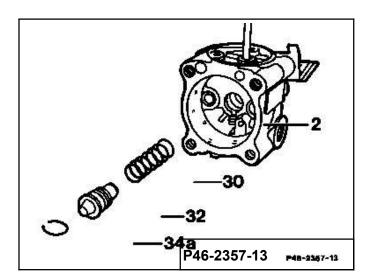
24 Clamp flow control valve (32) in a vise at a part which is not ground and unscrew valve screw (53) of the overpressure valve.
