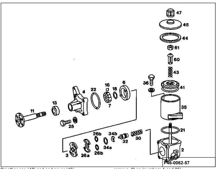
Breather cap (47) and end cover (45) remove, fit on (numbers 1 and 25).
