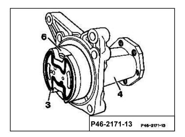
23 Insert O-rings in bearing flange, then insert bearing flange (4) in the pump housing and attach with the hexagon bolts (25). Tightening torque 30-35 Nm.
