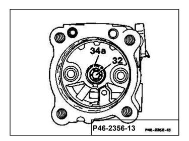
23 Take flow control valve (32) and compression spring (30) out of the pump housing (2).
