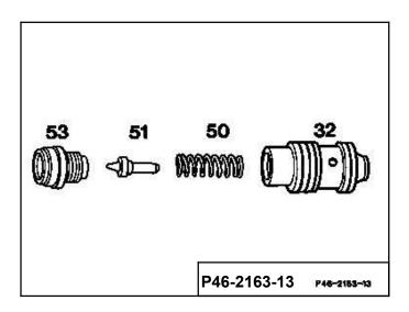
15 Insert compression spring (30) and flow control valve (32) into the pump housing (2).
