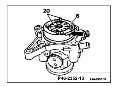
40 Fit pressure plate (3) with the ground face pointing toward cam insert (6).
