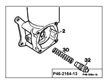
12 Clamp flow control valve (32) in a vise at the part which is not ground, and unscrew valve screw (53) of the overpressure valve.
