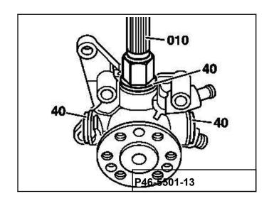
11 Check seals (39), replace if necessary. Take piston (37) and spring (38) out of the screw cartridge (40). Examine piston and piston track for signs of damage and wear. It must be possible to move the piston in the screw cartridge (40) easily and without it jamming. If this is not the case, replace the screw cartridge.
