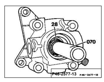
28 Press spacer ring (27) into the housing (4) with groove facing seal.
