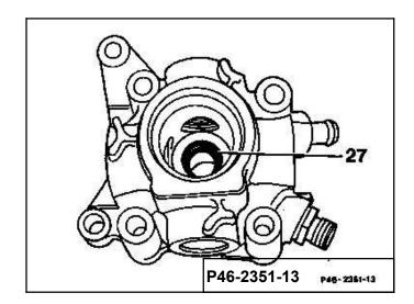
21 Pull out radial seal ring and washer (28) with internal extractor 000 589 33 33 00. Examine bronze bush in housing (4) for signs of damage and wear, replace housing, if necessary.
