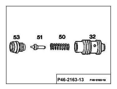
25 Check both sealing cones (high-pressure expansion hose, return pipe connection). Replace misshapen sealing cones. This is done by cutting a thread with M7 or M10 a few thread turns deep into the sealing cone. Withdraw the sealing cone from the housing with an M7 or M10 bolt. Fit on new sealing cone in housing and press into the housing by screwing in the high-pressure expansion hose or the return pipe.
