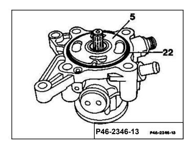
36 Fit rotor onto the drive shaft so that the chamfer on the inner diameter (arrow) is facing the thrust washer.
