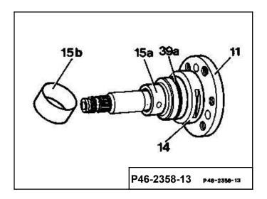
32 Carefully insert drive shaft (11) together with bearing flange (14) into the housing (do not damage seal). Ensure that the groove for the roll pin (19) is parallel to the roll pin bore. Knock roll pin (19) into the housing.
