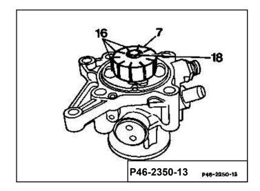
Detach rotor (7) from the drive shaft (11) with a plastic-headed hammer and take off together with the vanes (10 off). Check the vanes (16) in the grooves of the rotor (7); they must slide easily in the rotor.
