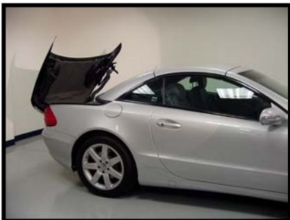
Top sequence: Opening Top operates until pictured. Pump continues to run.
