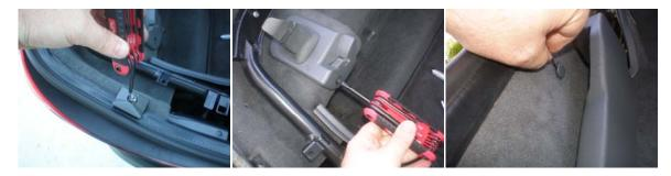
Step 3- Pull back the carpet out from underneath the weather stripping so you can get at the nuts. You will also need to remove the panel and small plastic cover on the driver side to get at one of the nuts.
