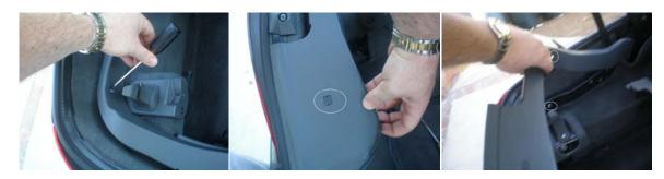
Step 2 – Unscrew the Star bolts for the carpet/weather strip and the trunk cover latch. You will need to keep the passenger side trunk cover latch connected to the electrical plug and intact so that when you partially open the top, the latch will be engaged to allow this function. There are a couple of plastic snap pins for the carpet that will also need to be removed.
