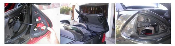
Step 5 - Pull out the light partially and disconnect the harness plug by pressing on both sides of the plug with your fingers.
