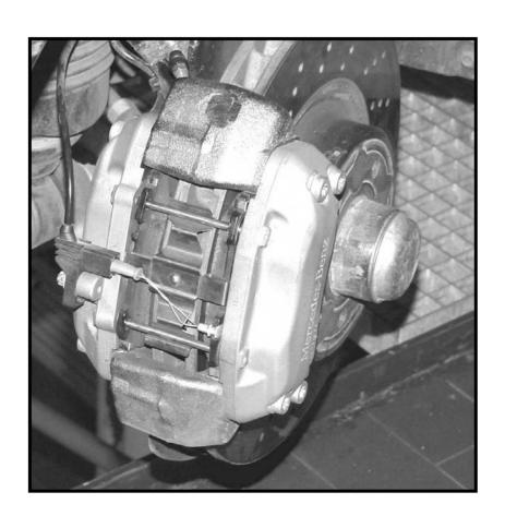
Three brake pad wear sensors connected to closest SAM
