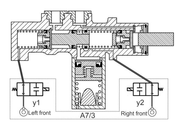
In the event of a SBC system failure the front brakes are braked hydraulically by the brake pedal without power assist.
