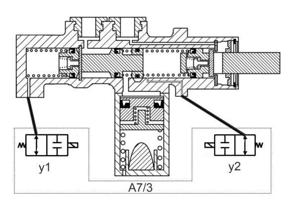
The outlets ports are connected to A7/3 (SBC hydraulic unit), which contains separation valves y1 and y2.
