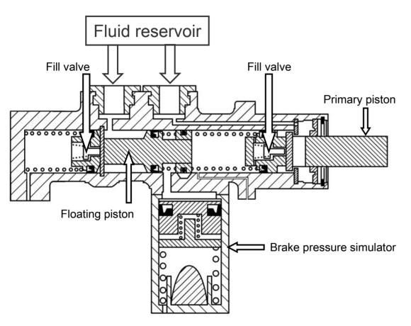
The fill valves open against the small spring pressure, allowing the fluid from the reservoir into the body of the master cylinder.
