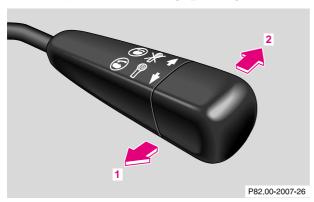
The operating lever for the voice recognition system is located on the right side of the steering column.
