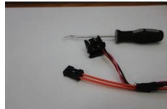
1c. Fiber optic cable removed from the factory radio plug
