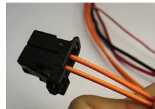
1d. Optics installed in the provided outer coupler
