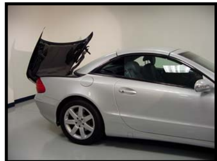
Top sequence: Closing Top operates until pictured. Pump runs for about 10 seconds longer, then stops.
