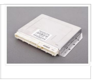
Now if the control module senses inadequate pressure to operate, or if any of the sensors provide in-plausible data, the system will shut itself down for safety reasons. The o ending sensor will be logged for later retrieval by the SDS system.
