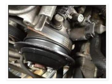
The power steering and ABC pump are integrated into one unit, referred to as a Tandem Pump. Although the two pumps share the same pulley and shaft, they are separate components otherwise. It is possible for the ABC pump to fail but the power steering pump is fine (and vice versa). But if one fails, both have to be replaced since they are one unit.
