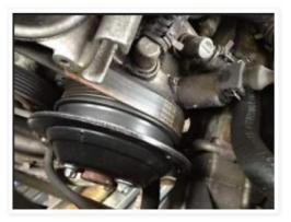
The power steering and ABC pump are integrated into one unit, referred to as a Tandem Pump. Although the two pumps share the same pulley and shaft, they are separate components otherwise. It is possible for the ABC pump to fail but the power steering pump is fine (and vice versa). But if one fails, both have to be replaced since they are one unit.
