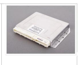
Now if the control module senses inadequate pressure to operate, or if any of the sensors provide in-plausible data, the system will shut itself down for safety reasons. The o ending sensor will be logged for later retrieval by the SDS system.
