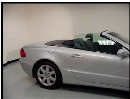
Top sequence: Opening Top operates fully except pump continues to run - warning tone rings and windows never fully close - 1/4 inch gap remains.
