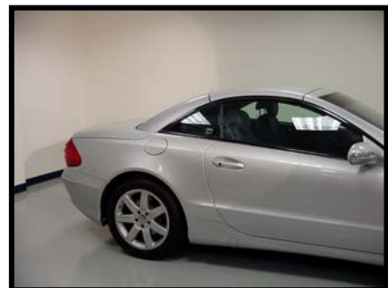
Top sequence: Closing Top operates fully except pump continues to run - warning tone rings and windows never fully close - 1/4 inch gap remains.
