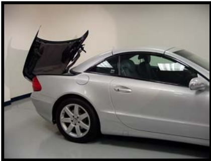
Top sequence: Opening Top operates until pictured. Pump stops, will not reverse - STUCK.
