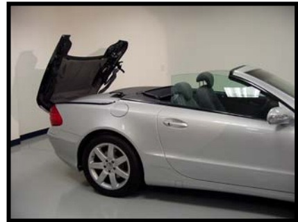
Top sequence: Closing Top operates until pictured. Pump stops, will not reverse - STUCK.
