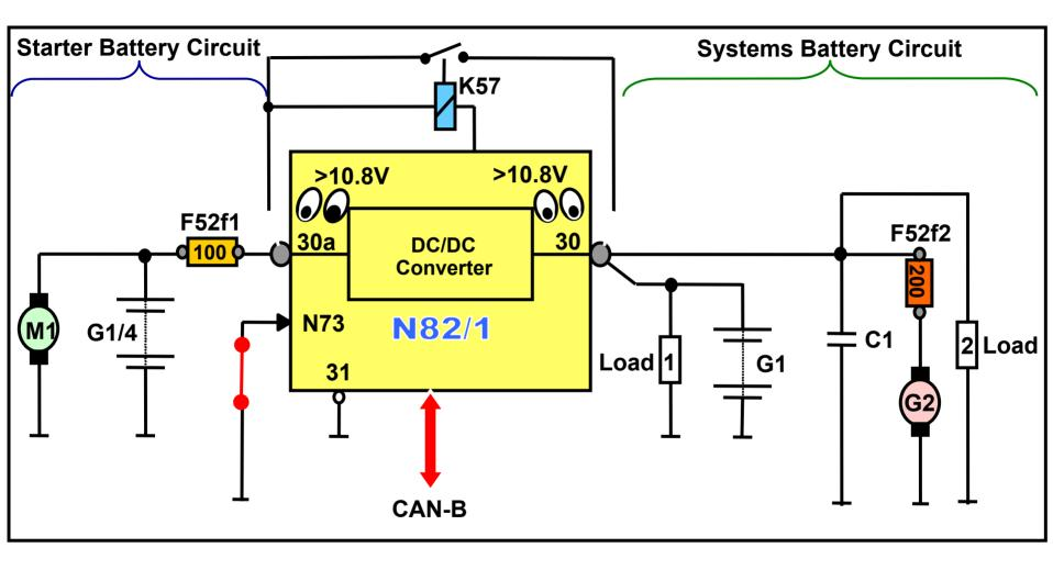
N82/1 control module checks battery voltages
