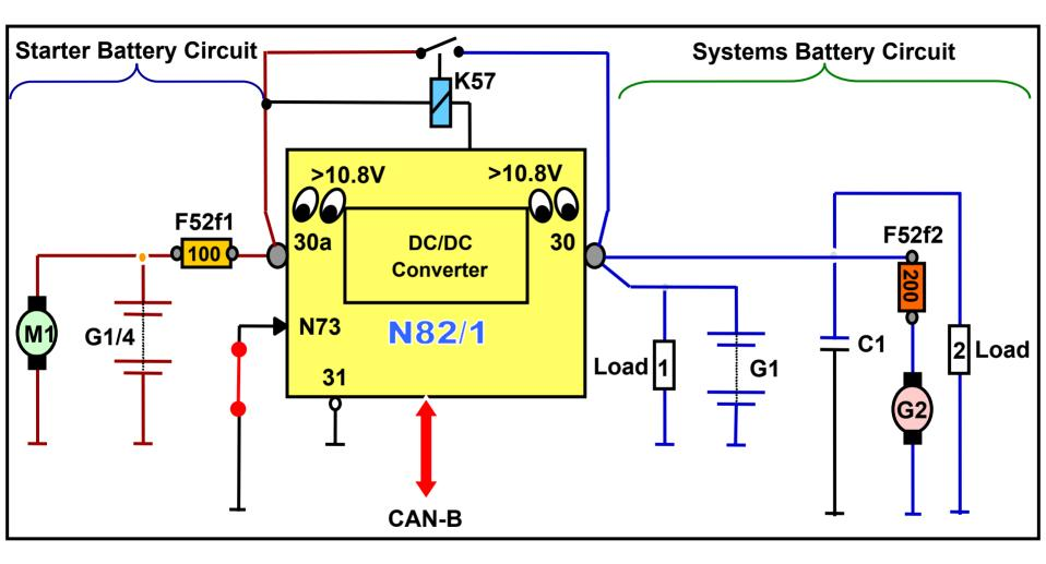
N82/1 control module isolates starter battery from systems battery via open relay K57 (not energized)
