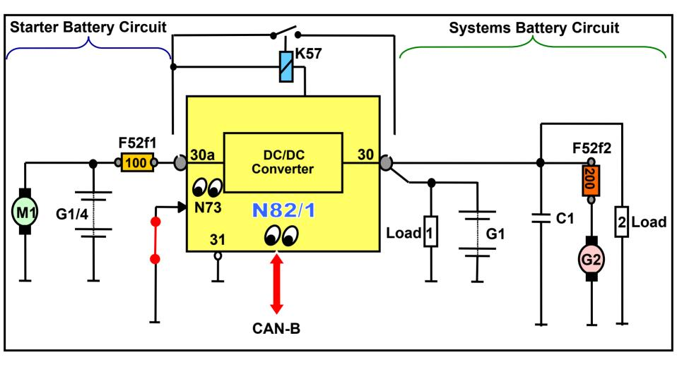
N82/1 control module is activated by: CAN-B or microswitch in EIS
