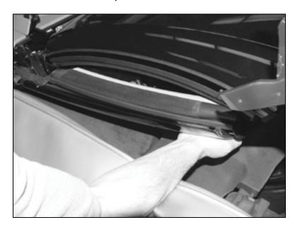
10. At this point, readjust your hand to firmly pull up on the bottom of the C-pillar. You **MUST** keep upward pressure in this area during the entire raising process. Failure to do so will cause the rear hat shelf and rear window to contact as well as the roof will not line up with the locks in the crossmember (windshield header) and may cause damage to the roof or weather stripping.
