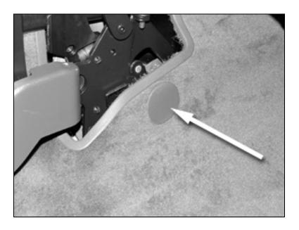
4. Using a 6mm Allen wrench, unlock the tubular frame locks.
