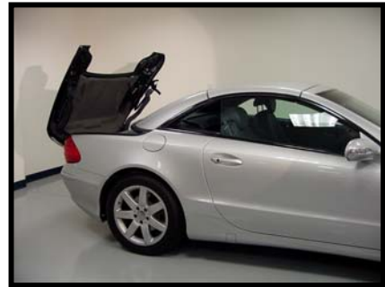
Top sequence: Closing Top operates until pictured. Will not reverse. - STUCK
