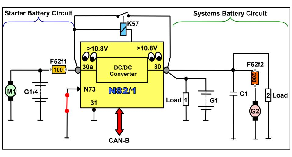
N82/1 control module checks battery voltages
