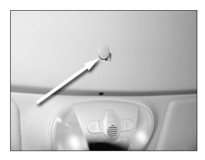
13. With the roof locks unlocked, move the roof forward to insert the right and left lock mounts into the crossmember (windshield header) and lock the Vario roof. **Counterclockwise to lock**.
