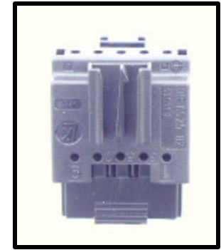
Bridge cover pulled up disconnecting wake-up lines
