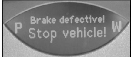
If the SBC system shuts down, you default to the emergency braking mode, all vehicle speed related functions may also stop depending on the failure. Certain faults will trigger an audible signal.
