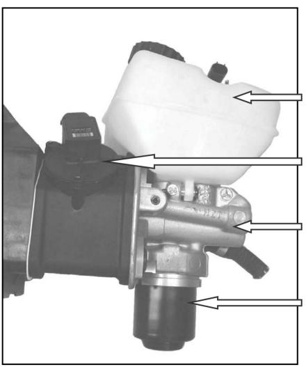
The Brake Operating Unit (BOU) consists of the following:
