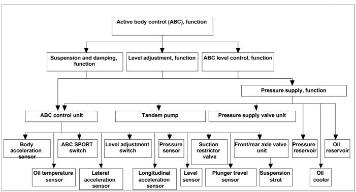
Active Body Control (ABC) is an active suspension and damping system. The entire static and dynamic load is handled by the four suspension sturts located at the wheels. Each suspension strut has a dynamically adjustable hydraulic cylinder (plunger) fitted in series to a coil spring and in parallel to a shock absorber. The hydraulic cylinders move to produce forces that counteract wheel movement.
