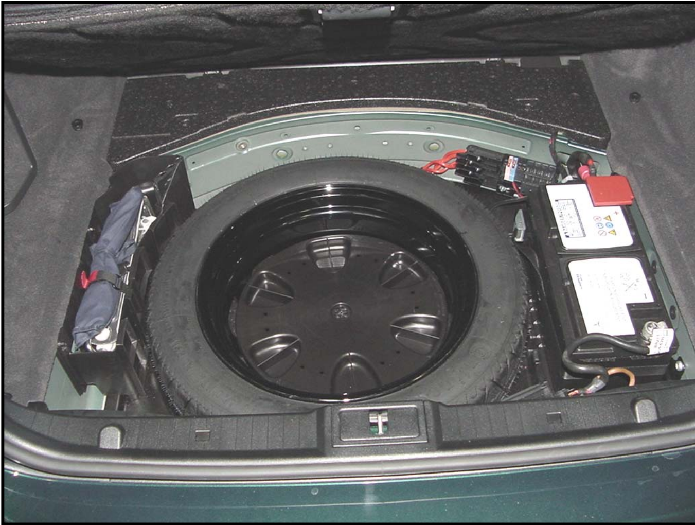
Location: (G1) installed in trunk
