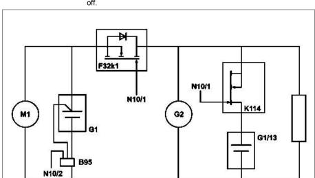
The additional battery relay for ECO start/stop function disconnects the additional battery for ECO start/stop function from the on-board electrical system. The energy requirement of the on-board electrical system is now supplied again by the on-board electrical system
