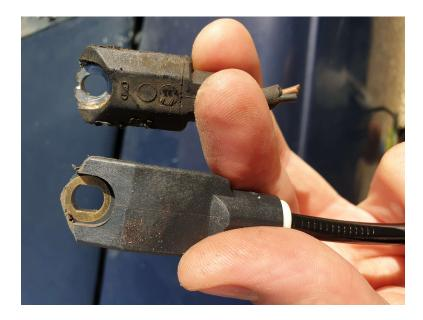
Once installed it works perfectly, with the ABS light coming on at ignition and staying off after. I haven't tested it on ice/emergency breaking yet(!), but understanding the physics of these sensors there is no reason it shouldn't work to engage the ABS, and in any case it must be outputting a reasonable wheel speed sine wave to the ABS computer otherwise the light would come on.
