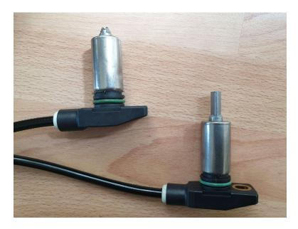
You should be careful to cut the groove in the tip to match the original \*perpendicular\* to the axis of the sensor head.
