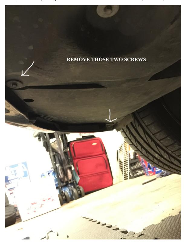
Then, take the front passenger side bottom cover off. Use the Wrench in the picture or equivalent tools.
