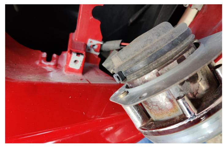
You may have to use snips to cut the zip tie to be able to remove the gasket. Once you've done this and pulled back the gasket remove the 2 wire connectors where Black is Top and Red is Bottom
