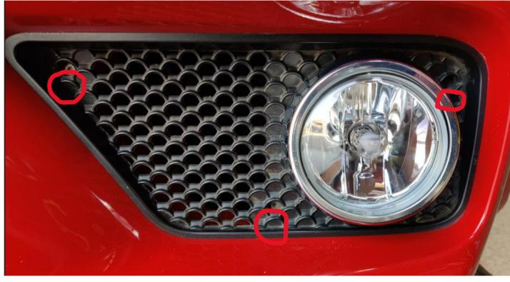
Next after removing the 3 screws is to remove the black mesh screen where the fog light bezel is part of the screen. You know have access to remove the fog light assembly where there are 4 T15 Torx screws in each corner to be removed
