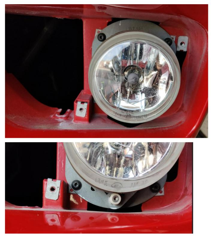
After removing those 4 T15 screws pull the light assembly out exposing the wire connection. Your fog light more than likely has a rubber gasket protecting the wire connections, just pull back on the gasket to expose the 2 wire connections.
