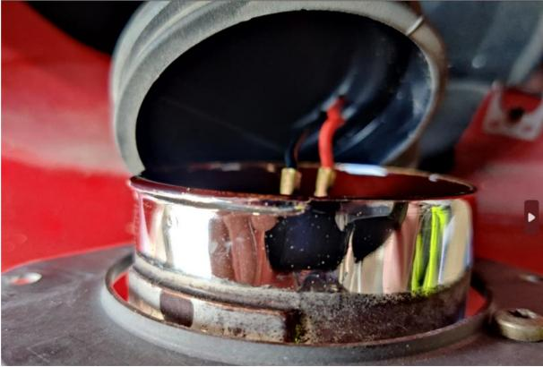
After removing those connections the assembly comes off. Next you'll want to make sure the new light adjust is the same as your old one by lining up the assemblies and make the corre sponding adjustment to the new light via the adjustment screw:
