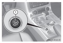
Trunk Wing switch ① should be used for cleaning only, see "Trunk Wing" (▷ page 360). It is not needed for Trunk Wing operation.
