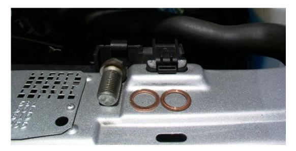
When the drips have slowed sufficiently, fit a new gasket and reinstall the drain plug, tightening securely. Since you should have your torque-wrench handy anyway for the filter housing, you may as well torque it. 20 lb/ft is sufficient.
