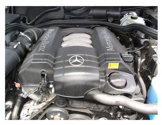
This cap-style filter wrench has a 3/8" square drive, so connect a ratchet and short extension and just loosen it and keep loosening. The o-ring will usually make it feel pretty tight until it's almost completely unthreaded. Have two clean, lint-free rags handy before you lift it out, one to catch any drips and the other to cover the hole so no dirt (or tools or parts!) can accidentally fall in. The latter will definitely ruin your day and your wallet.
