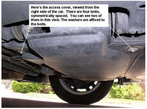
When you remove the cover...you'll find that drain plug. You'll need a 13mm wrench or socket to remove it. Have a LARGE drain pan handy, you'll get more than 2 gallons of oil out. Note that the placement of the plug towards the middle of the side means if you lift the front of the car, oil will pool in the back of the pan and you're not really changing the oil, just diluting it.
