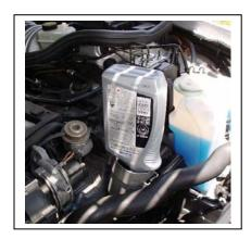
When you get to the last quart pour half of the quart into the filter assembly hole (there's a little translucent window on the edge of the oil bottle that is marked with gradation lines) and then pour some oil in the cap you set aside until the cap is about 1/2 full. Re-cap the 1/2 bottle so it stays clean. At some point and certainly by a few thousand miles you'll need it to top off the oil.
