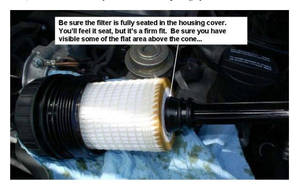
Toss the three smaller O-rings in the cap of oil, and then dip your (clean!) fingers in to get some oil and use it to lube the largest O-ring. Slide it up the assembly and seat it in the groove above the threads. Now install each of the other O-rings, in size order, with the next largest down to the smallest.
