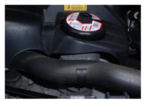
Pull the entire filter assembly out, keeping it straight until the last of it clears; it extends down into the engine more than a foot. It's pretty durable, but it's composite, so don't manhandle it: I can't imagine it's inexpensive to replace. Plus fishing pieces back out of there would definitely NOT be fun. If you wish you can wipe some of the old dirty oil out of the inside of the filter hole before you cover the hole up. Once the assembly is out, here's what it looks like.
