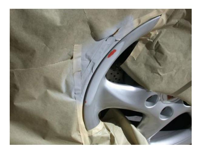
Okay, here's where a bit of laziness is going to create an entire new clay-bar project. This metallic paint will GET EVERYWHERE. I'm talking permanently attached to the fender on the opposite corner of the car...mask CAREFULLY and COVER THE WHOLE CAR with a sheet or equivalent.
