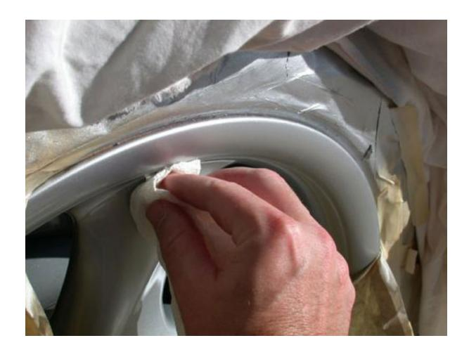
AND here's the nicely painted wheel. I'm going to not be an idiot and let the paint dry OVERNIGHT (like I knew I should) and do the clear coat and I'll post that tomorrow.
