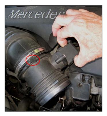
Holding the clip firmly, rock the assembly and connection while pulling the connection away from the assembly. With the electrical connection unplugged, it is now very simple to remove the assembly. Note the little alignment tang/ear on the intake side of the assembly; in the shot above it is deflected so it's easier to spot.
