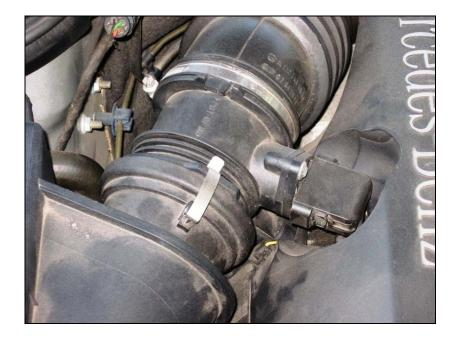
Three things fix the MAF assembly to the vehicle: two clips on the airbox side, a worm-gear type clamp on the intake side and the electrical connection. In the above shot you can see the latter two very clearly as well as one of the two spring clips.
