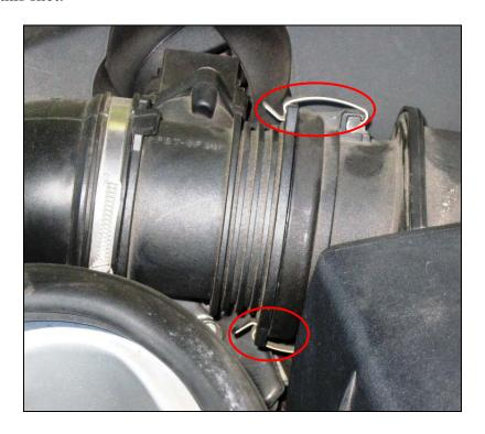
With the airbox cover removed you can see the MAF assembly a bit better...
