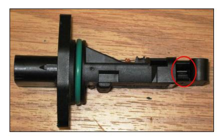
This shot shows one angle for the straw on the MAF aerosol cleaner. The metal surface to be cleaned is a bit more visible from this aspect.
