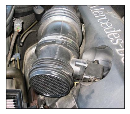
Loosen the worm-gear clamp with either a screwdriver or a 7mm nut driver. Do NOT remove the assembly at this point or you will put undue stress on the wiring. While you
