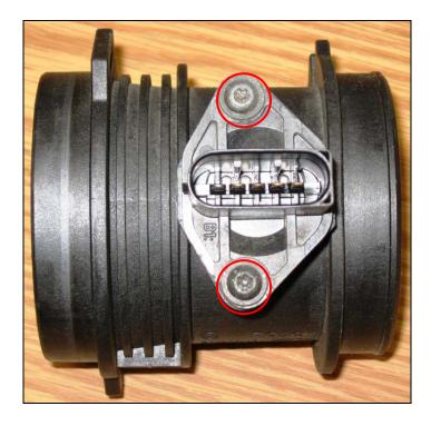
With the screws removed, rock, twist and pull to remove the sensor from the assembly:
