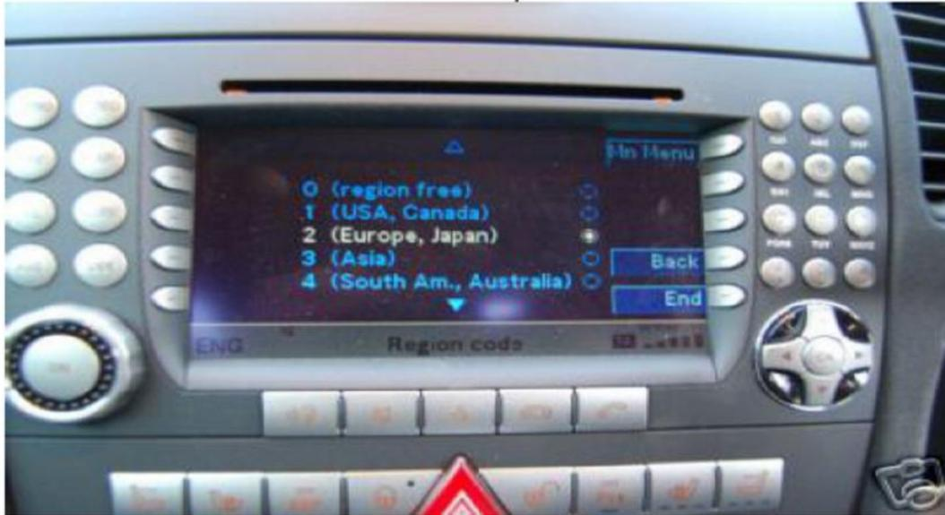
Using the arrow keys, highlight the region free setting and enable it using the **OK** button.
