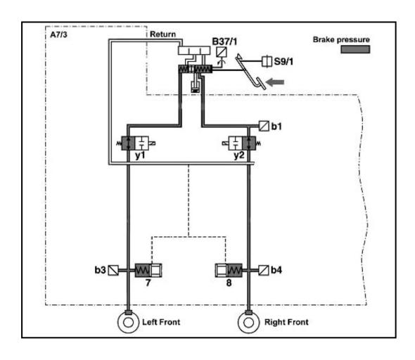
A7/3b1, b3, and b4 are pressure sensors that provide information to the SBC control module.
