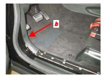
Carefully pry the holding brackets with an wedge or with a wide slot-head screwdriver out of the lateral covering in the foot well (b). The covering is locked into a holding bracket at the car body in the region of the fixing brake. Remove the covering.
