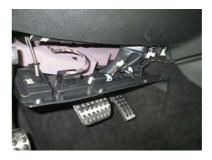
Unscrew the nuts of the accelerator. Lift out the accelerator and pull off the connectors.
