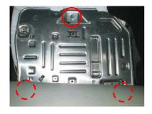
Flap the fastening plate in the direction of the passengers seat to get to the control unit AIRMATIC.
