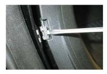
Unscrew the screw of the engine hood release (c). Unscrew the 3 screws of the lower cockpit covering in the driver's foot well.
