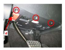
Take down the cockpit covering. Hang out the cable winch of the engine hood release. Unlock the diagnosis coupler and push it upwards to remove it. Remove the connector of the foot well light and remove the air pipe. Take out the cockpit covering.
