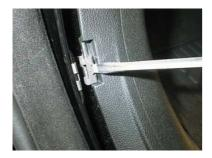
Pull off the covering of the slide rails (b) by inserting an adequate tool into the slot to release the covering.
