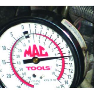
This engine was generating too much boost from a Recirculation Air Flap actuator that was sticking closed. The engine started missing as injectors were being shut off and timing was being retarded.
