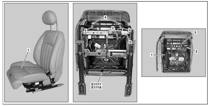
Shown on front passenger seat1Seat cushion2Seat occupied recognitionconnector(front passenger seat only)
