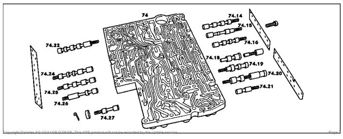
74 Valve housing 74.14 Command valves "1-2" and "4-5"
