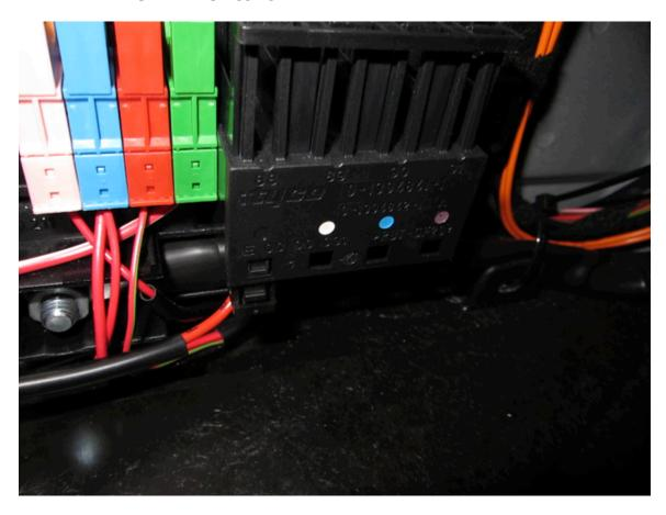
4. Find connection D on your harness – plug has 4 pins only 2 of which are occupied
