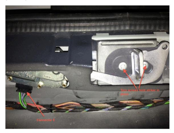
The way it functions is that when you press the button to close the trunk, the striker eye moves to the up position while the motor closes the trunk lid. The trunk closes onto the striker in the up position and pulls it down.
