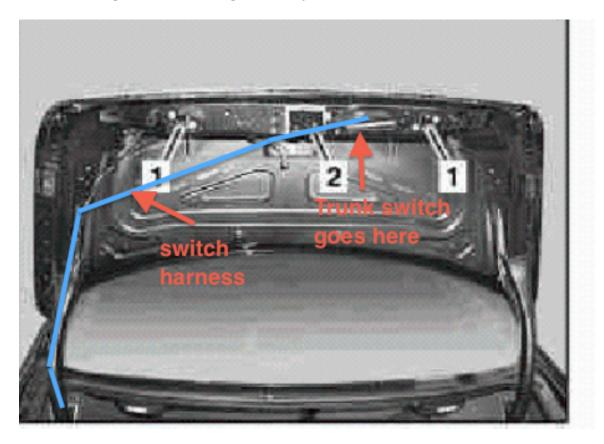
c. replace the trim after tip-tieing the cable in place
