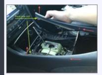
connect wires back, start the car shift in N or D and take out ashtray holder. Shift back in P and maybe disconnect rear battery.
