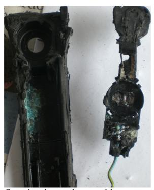
Corrosion also attacks some of the copper tracks
