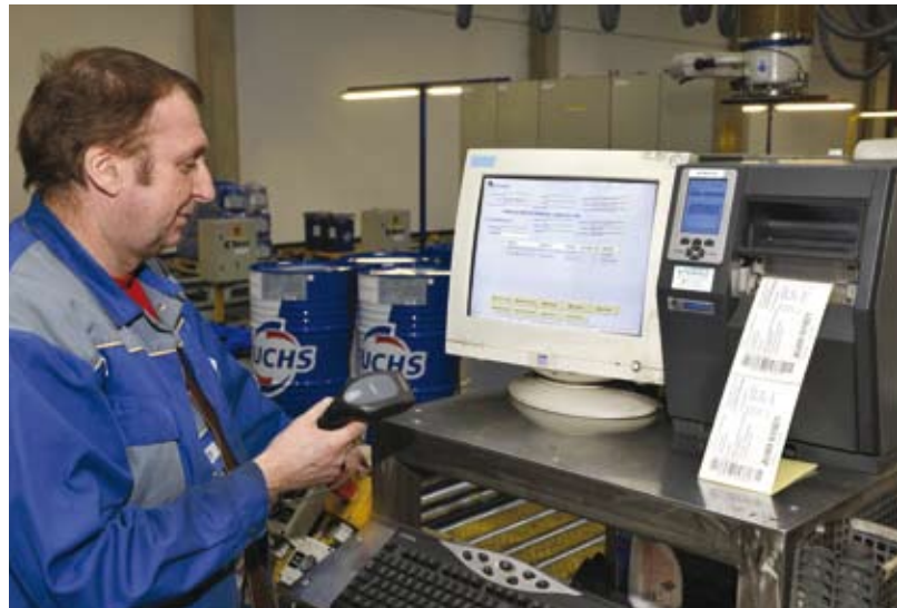
For each container, Jürgen Mädler prints a label comprising all logistics processing information by "docking" the pallet at the picking work station.
