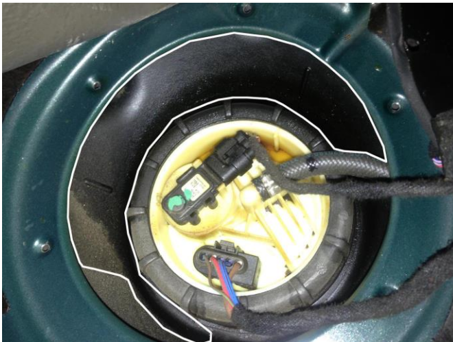
Figure 3 (Fuel residue outlined)
