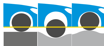
Active air suspension module based on "Skyhook" philosophy.
