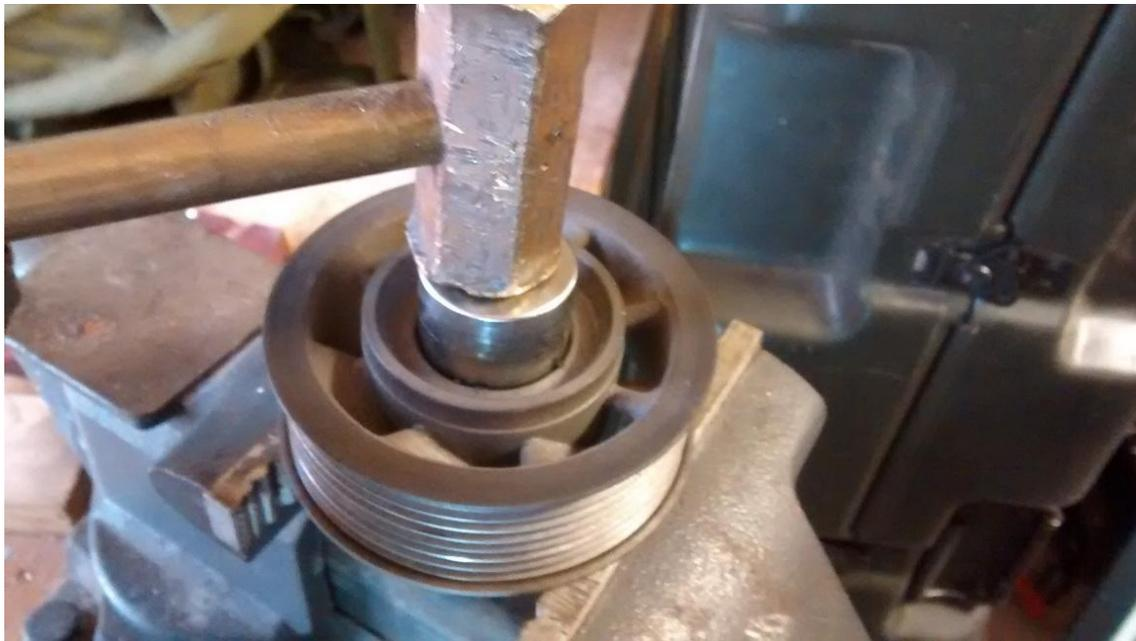
Use 24mm socket and hammer to finish tapping out the bearing.
