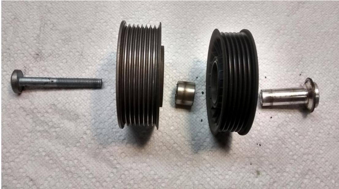
Separate the assembly. Note orientation of the aluminum pulley; circlip side is towards head of bolt.
