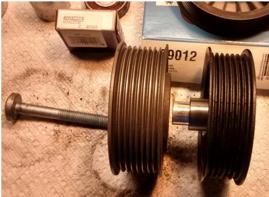
Reassemble the idler pulley.
