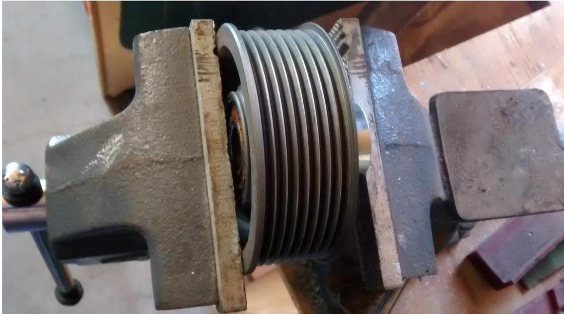
Use 24mm socket and vise to start pressing out the old bearing.
