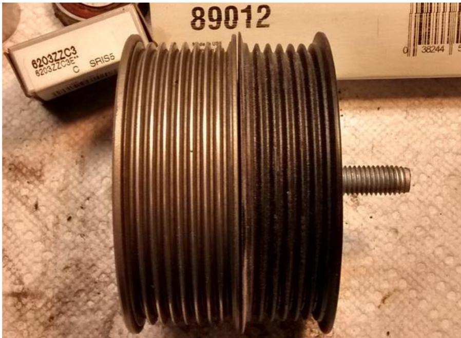
Note the small gap between the two pulleys. Ready to re-install on the car.
