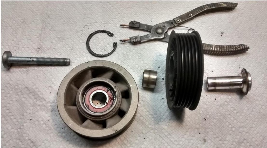
Remove internal circlip.
