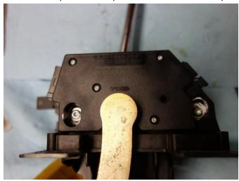
Remove the two torx screws, slide module away from the chrome shift lever, and lift off. I recommend you have the chrome shift lever in neutral position to make this easier. Do not force or you can break the tabs to the position sensor!
