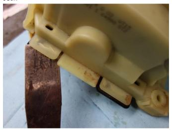
Lift upper shell and remove connector to the +/- side-shift switch.
