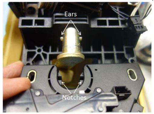
Installation is literally the reverse of removal. I applied a light coating of silicon seal to glue the upper and lower shift module shells together immediately before bolting down. After the bolts are torqued, the upper and lower shells are held tightly together. With the upper black access cover removed, you can easily use a pair of needle-nose pliers to reconnect the electrical connector for the +/- side-shift switch and then reinstall the upper access cover.
