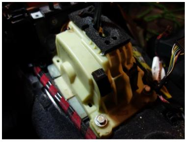
Lift shift module, tie shift rod up with mechanic's wire (or a coat hanger) to prevent the shift rod from dropping into the transmission tunnel. Remove clip (don't drop it!), and slide shift lever and bushing off of the shift rod. Note I did not follow the last instruction; leave the bushing in the end of the shift lever as it is a PITA to reinstall the bushing into the shift lever!
