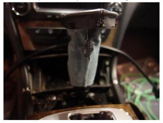
Twist locking nut to release. Lift shift knob straight up; do not twist!
