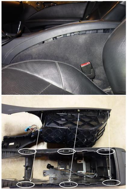
Move ashtray out of the way by releasing two tabs with a small screwdriver. This photo is out of sequence; the two inner screws should still be in place at this time. I had already removed the two inner screws and realized I could not remove the lower half of the console until I moved the ashtray out of the way.
