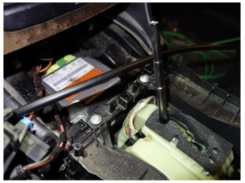
Remove two screws at rear and disconnect electrical connectors:
