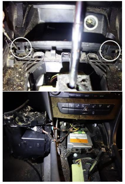
Remove the two inner screws at the front:
