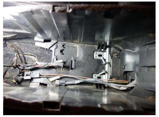
Lift front of console to release the "tabs and slots" from the center dashboard and remove lower half of console:
