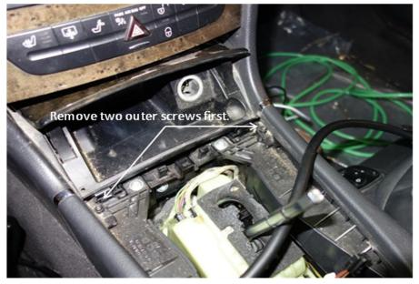
Remove upper half of console by lifting straight up. It is held in place by six each metal clips that fit into plastic fittings in the console bottom.
