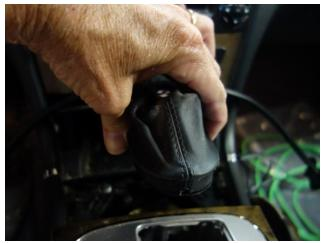
Pull boot upward to expose the locking nut on the shift knob:
