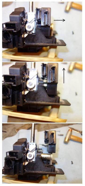
The two ears fit into the two notches to mate the shift lever axle to the shift position sensor.
