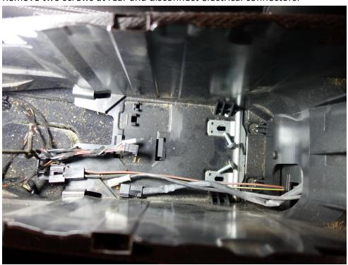
Lift front of console to release the "tabs and slots" from the center dashboard and remove lower half of console:
