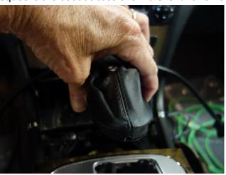
Pull boot upward to expose the locking nut on the shift knob:
