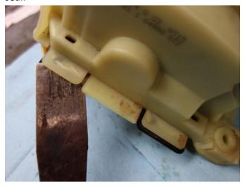
Lift upper shell and remove connector to the +/- side-shift switch.
