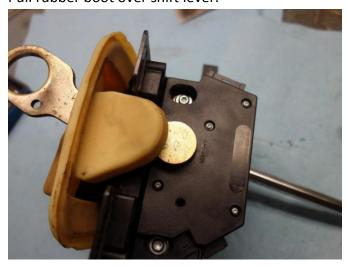
Mark screw position so you can match the new part to the old calibrated position.
