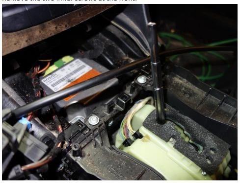
Remove two screws at rear and disconnect electrical connectors:
