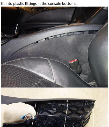
Move ashtray out of the way by releasing two tabs with a small screwdriver. This photo is out of sequence; the two inner screws should still be in place at this time. I had already removed the two inner screws and realized I could not remove the lower half of the console until I moved the ashtray out of the way.
