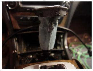
Twist locking nut to release. Lift shift knob straight up; do not twist!
