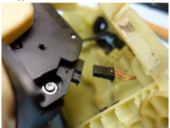
To reinstall that connector later, remove the plastic access cover on the upper shell.
