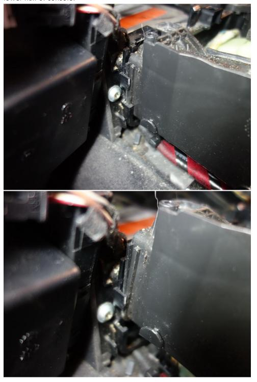
Remove three bolts holding shifter module to the transmission tunnel. There are three electrical connectors in the front plus a cable; release the cable by pushing down on the plastic tab and rotating the metal fitting 90 degrees. Cable fitting is "righty-tighty, lefty loosey", so rotate CCW to release. Remember, it is reversed when sitting in the car so rotate the top of the fitting towards the door on the right-hand side of the car. There is not much room there.
